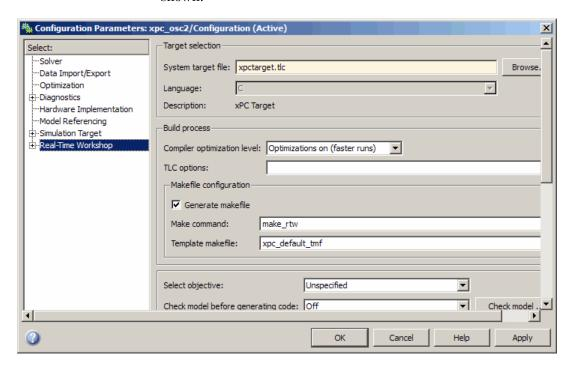
If you have the Real-Time Workshop Embedded Coder, you can build an ERT target application. To build an ERT target application, in the **Target selection** section, click the **Browse** button at the **System target file** list. Click xpctargetert.tlc, and then click **OK**.
