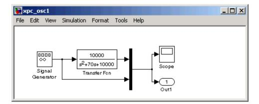
2 In the Simulink window, from the Simulation menu, click Configuration Parameters.
