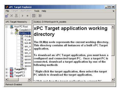
5 In xPC Target Explorer, check that the DLM(s) node in the xPC Target Hierarchy has the pathname of the folder that contains the prebuilt target application you want to download to the target PC.
