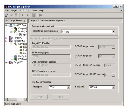
You do not have to exit and restart MATLAB after making changes to the xPC Target environment, even if you change the communication between the host and target from RS-232 to TCP/IP. However, you do have to recreate the target boot disk and rebuild the target application from the Simulink model.
