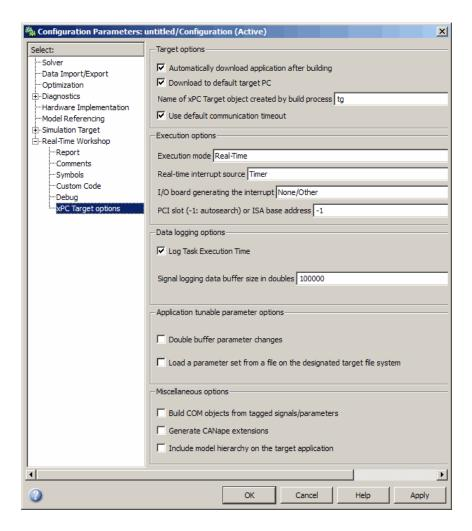
Automatically download application after building — Selecting this option allows Real-Time Workshop to build and download the target application to the target PC. If you do not select this check box, Real-Time Workshop builds the application (DLM), but does not download it to the target PC. By default, this check box is selected.
