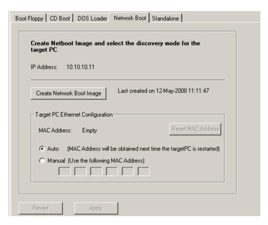
The **Target PC Ethernet Configuration** section of the configuration pane allows you to either associate a physical target PC MAC address with the xPC Target Explorer target PC name, or allow the software to automatically find target PC MAC addresses. If you want to associate your physical target PC MAC address,
